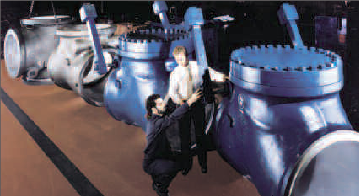
44" Cold Reheat Check Valves
