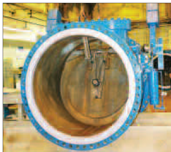
Compressor Check Valve with Oil Dashpot
